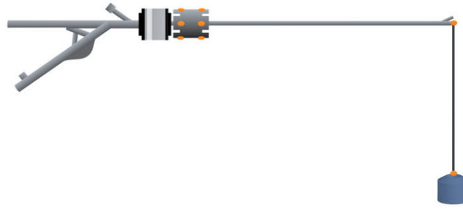
Figure 6. Needle driver, string, and weight used during the calibration procedure to align the template and force coordinate systems. Orange ellipses indicate the location of optical markers.
