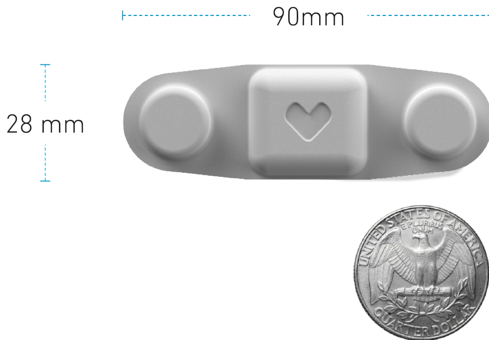
Figure 4.3: VIVALNK wearable ECG device [40]
